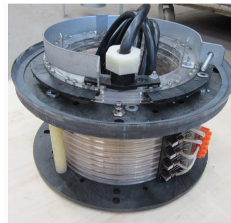
Collector Ring 集电环
