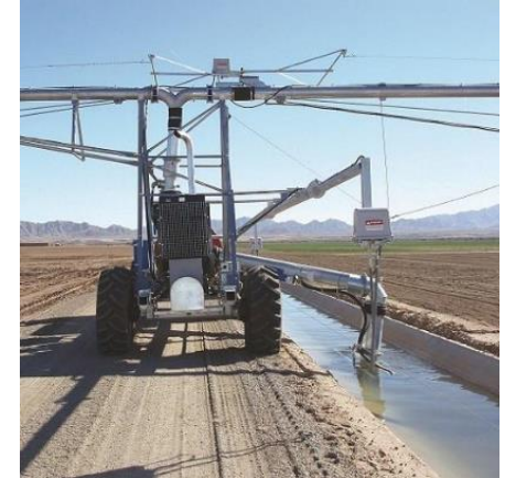
4-wheel Linear Move Irrigation System 4轮平移式喷灌机
