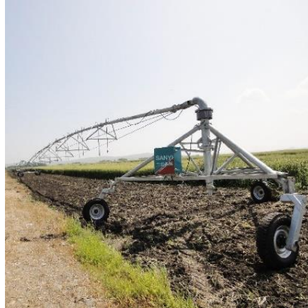
Towable Irrigation System 牵引式喷灌机
