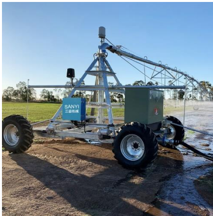
Linear and Rotating Irrigation System 平移回转喷灌机
